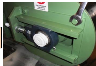
Fig.13- Removing the slide and support
