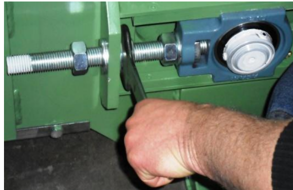
Figure 10 – Adjustment of the belt tensioners.
