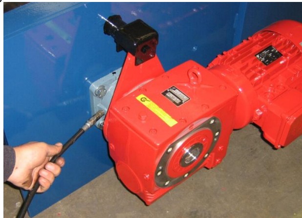
Figure 9 - Grease pair of front bearings
