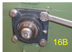
Fig. 16 – Removing support of the driver roller (A- gear motor side; B-side opposite to the gear motor).
